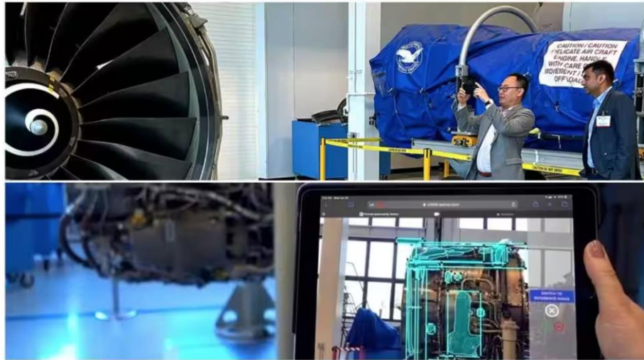
PW and Awiros team using the Percept Tool to scan a V2500 engine.
